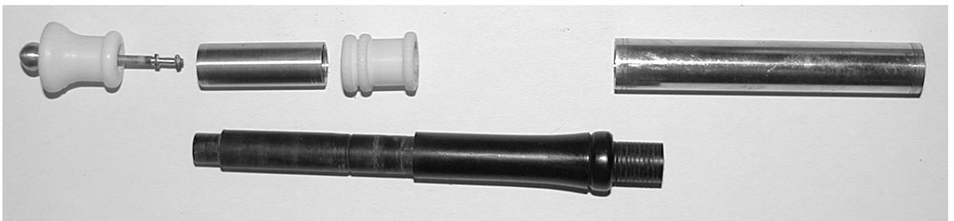
The sliding part may be turned and finished almost to completion using the tenon to grip in the lathe. The ferrule may then be glued on using heavy duty epoxy.
